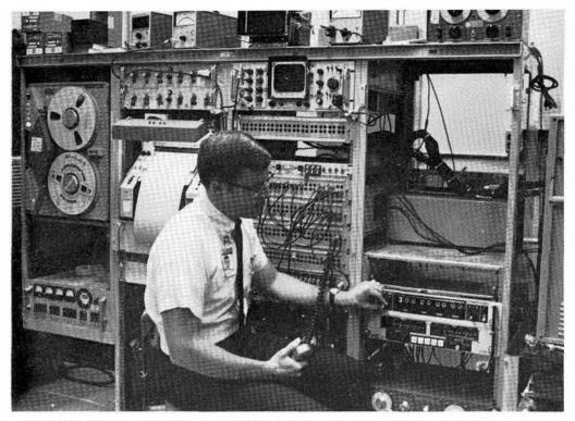
CONTROL POINT equipment, installed in a transporter for mobility, includes recorders, receivers, and other telemetering devices. Up to five buoys can be remotely controlled from a land or sea based command center. Jeff Gorin (7291) has responsibility for development of B-SHA.
